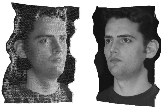
Figure 8 Face mesh recovered by C3D. Decimated polygon mesh (left) and photorealistic rendered model (right)
