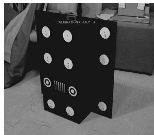
Figure 7 A calibration target with target circles located automatically
