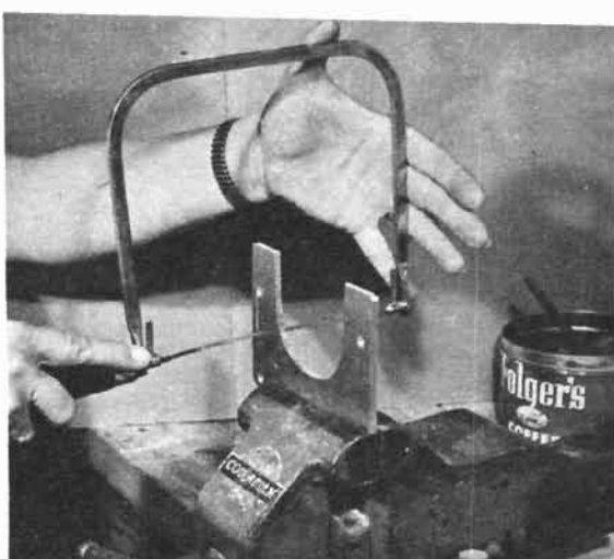
To cut slots in adjustable aluminum heel plates, drill holes and insert saw blade.
