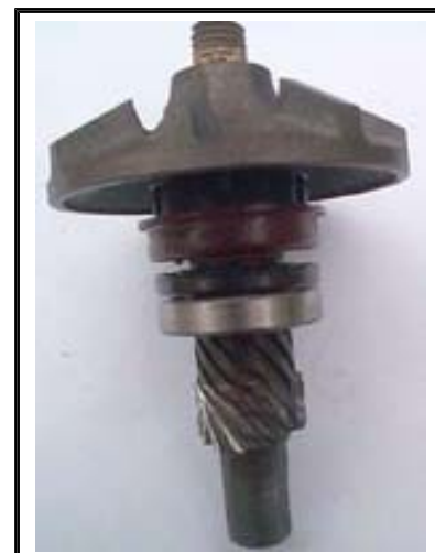
Original equipment water pump assembly showing stripped drive gears.
