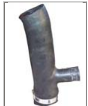
Stock 99 expansion tank hose modified by cutting off the curved end.
