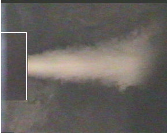
Figure 13 Visualisation of a non-vectorised primary jet for m_s/m_p = 0, dh/h = 0.04, \mathcal{A}h = 1, C_z = 0
