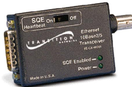
Figura 9.3 : Transceiver AUI/BNC
