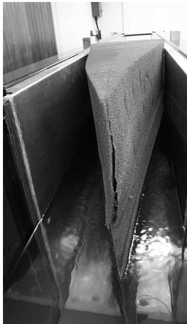
Figure 5.2: Picture of the triangular-shaped foam used to avoid wave reflection, fitted at the end of the wave flume.
