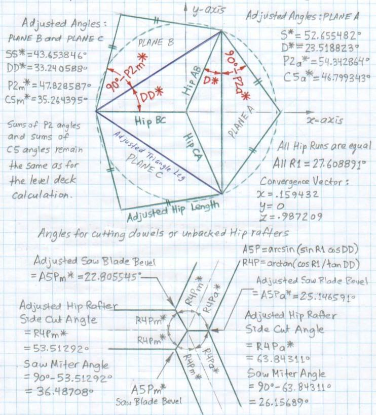
Development of Kite Angles Trigonal Trapezohedron (Cube) P2 = X = 450 Kite with two 90° corners 450 Tangent to diagonal =Hypotenuse of Plan Angle DD
