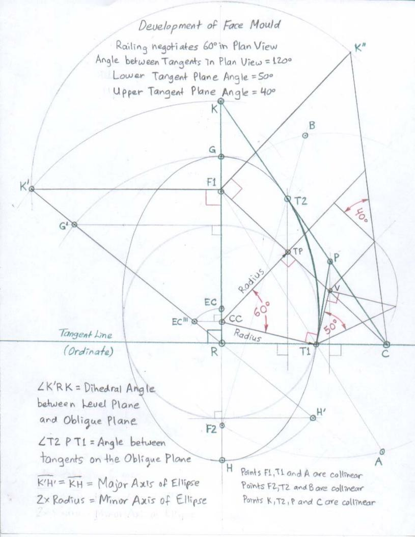
Construction of Twist Angles (Dihedral Angles measured between Tangent Planes and Obligue Plane)
