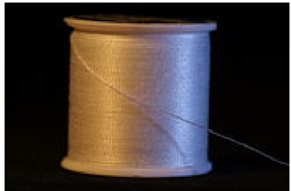
Spool of all purpose sewing thread, closeup shows texture of 2-ply Z-twist mercerized cotton with polyester core.
