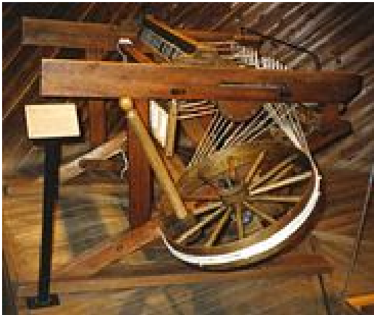
A Spinning Jenny, spinning machine which initiated the Industrial Revolution
