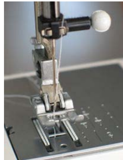
Needle plate, foot and transporter of a sewing
