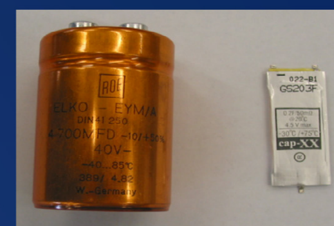
4.7mF electrolytic capacitor (left) Vs. supercapacitor up to 2F (right)
