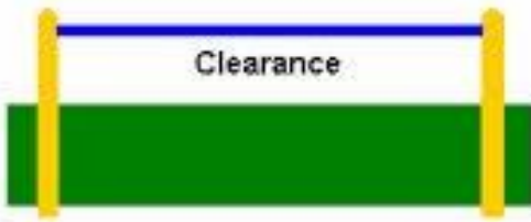
Figure 1: Clearance (In Air)
