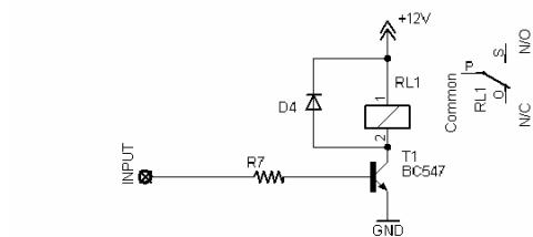
Eight such relay circuits are to be constructed to connect to pins RB0 to RB7 of IC1
