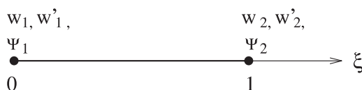
Fig. 4. The 2-node reference element of six degrees of freedom.
