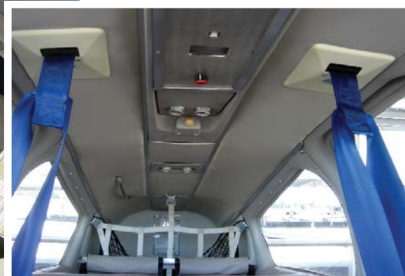
The BAS plastic escutcheons that fit around the headliner attach points, are a very nice finishing touch.
