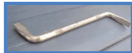
A 90° flat-bladed screwdriver is perfect for removing the retaining pins on the headliner.
