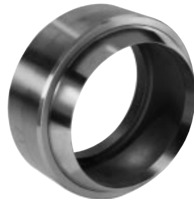
A helicopter swash plate bearing. The teflon liner in the I.D. of the outer race and the bore of the ball accommodates misalignment and linear motion.
