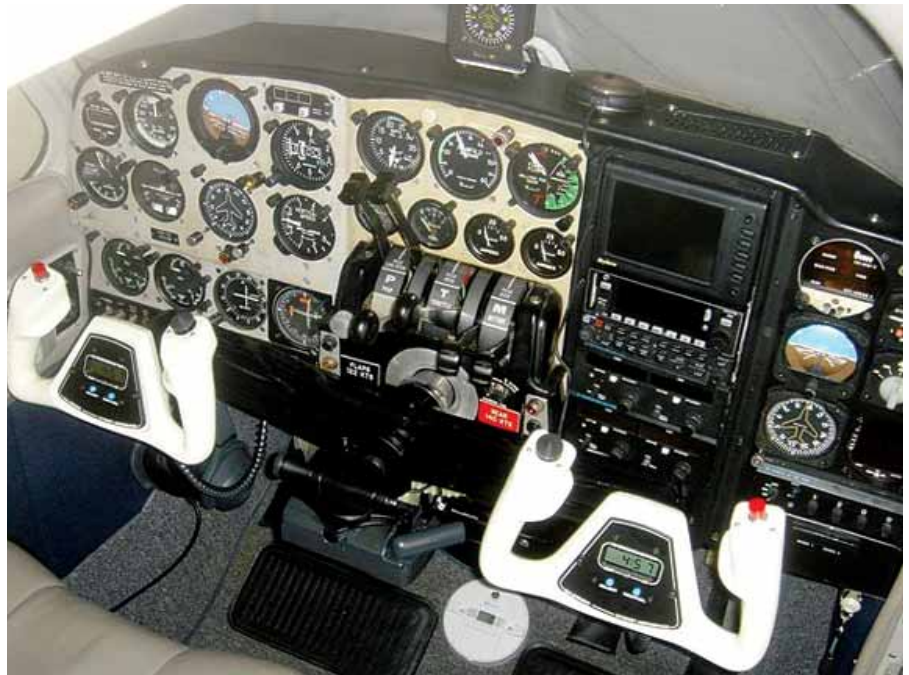
Fig. 9 - Full panel with GPSMAP in stowed position and GXM30 antenna in place on glareshield. No compass issues, since magnets were removed, via the procedure outlined by NUMA Aviation at http://www.numa.aero/GXM30.html
