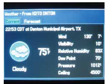
Fig. 6 - This is the "plain language" METAR interpretation that you get. Wind (speed and direction), visibility and ceiling. This works for me! By the way, this is exactly what is being broadcast at the time by ATIS/AWOS at the field.
