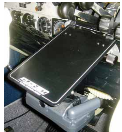
Fig. 5 - The GPSMAP when stowed with the flight desk in place for use.
