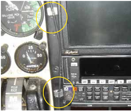
Fig. 7 - These clips from True Value Hardware keep the wires in place, eliminating dangling wire hell in your cockpit.
