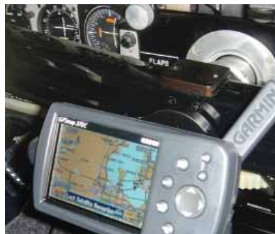
Fig. 3 - The unit with the flight desk removed from its mounting pedestal. In this position, I received plenty of satellites and had WAAS position accuracy of 9' within about 10 minutes.
