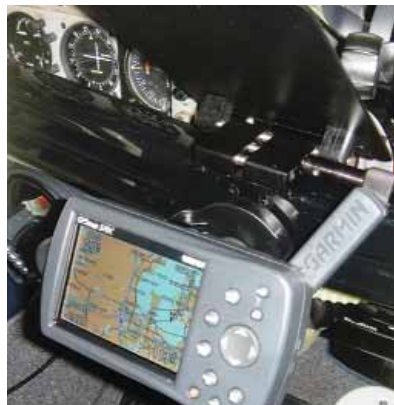
Fig. 2 - Place the marine mount with your GPSMAP onto the base disc that you just attached to the yoke. You can see the clearance available under the stock Cygnet flight desk.
