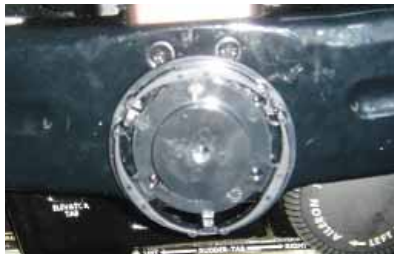
Fig. 1 - We started with the base of the stock Garmin marine mount. This base is mounted to the center of the yoke by removing the 12 o'clock position screw in the center circular plate. I replaced the short screw from the Cygnet yoke with a #8-32 x1/2" stainless steel screw and screwed the base of the Garmin marine mount in its 12 o'clock position to the yoke.
