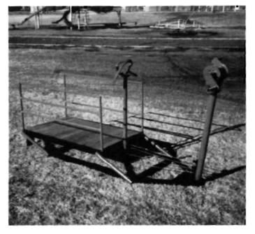
Construct a head catch using 1/2" diameter sucker rod and bend in the shape shown. To the base of the head catch weld a pipe 2"x 33".
