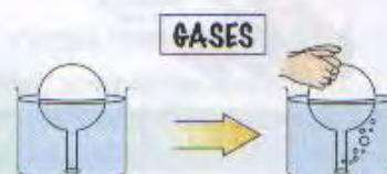
The gas inside the flask expands when it is heated by the warmth of the hands.
