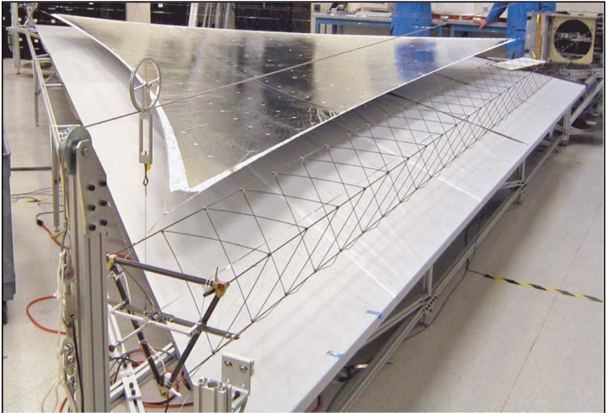
SAILMAST is the thin triangular truss in front of the picture. It is attached to a section of a silver foil solar sail section shown here in a laboratory test. The mast in the picture is 2m (6 ft) long. The Space Technology 8 mission will test the SAILMAST, which is 20 times longer.
