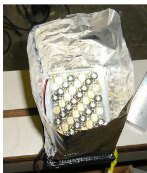
Figure 6.4. LED array covered with aluminium foil, to test the light intensity.
