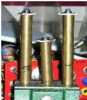
Figure 6.1. Design of the LEDs mounted on the poles, in order to test their light intensity.
