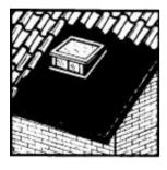
Modified Urethane Elastomer. A Cold applied liquid coating, Catalyst (Curing agent) added just prior to application.
