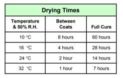
These times are based on recommended dry film thickness. High humidty, high film thickness or cooler temperatures will lengthen dry to handle/topcoat and final cure due to slower water evaporation rate.
