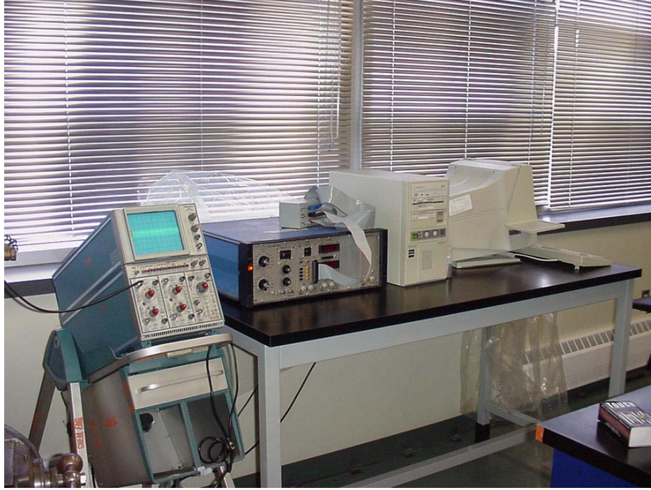
Figure 4.2e. A photograph of electronic components of an LDV
