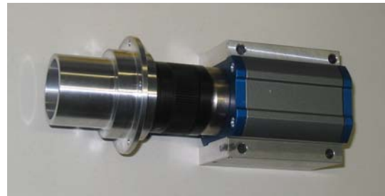
Figure 5: The 50 mm lens, Kappa camera, extra baffle and mounting system
