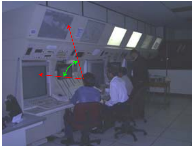
Figure 2. Knobs and switches located far from reaching causes duress postures and angle of seeing that is very large.
