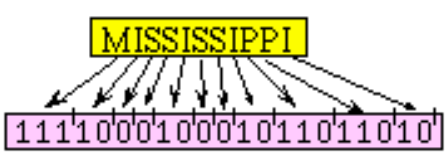
Figure 9-7: Huffman encoding for MISSISSIPPI
