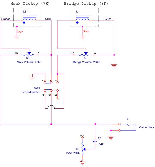
Fits in existing cavity and existing holes. No modifications to body or hardware required. Old volume controls can be reused. The Series/Parallel switch is a push-pull type part of the tone control R3.
