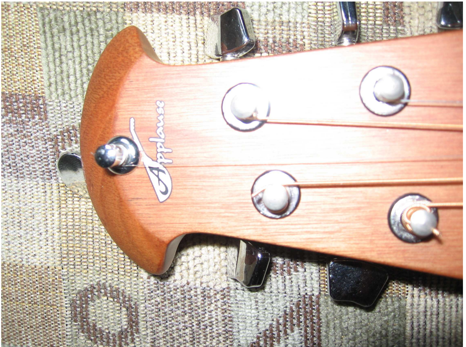
View of the top of the headstock showing the critical placement of the tuner shaft. If your headstock is not beveled, then obviously this becomes a non-issue.
