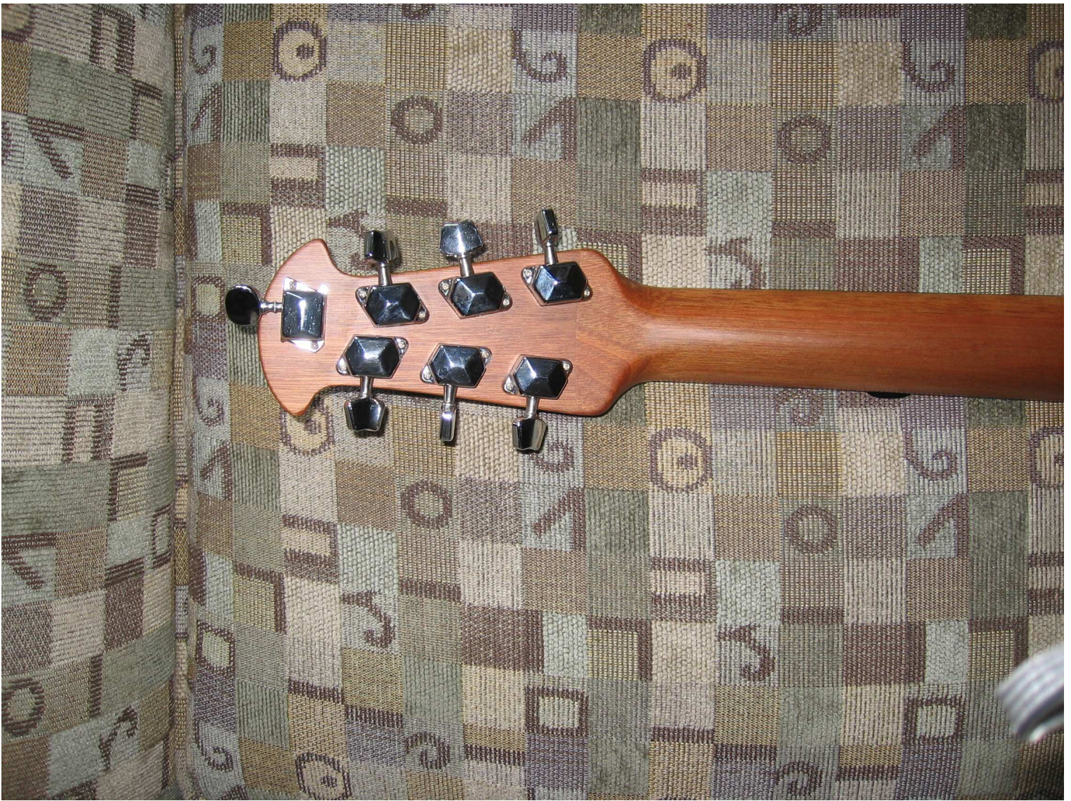
Here's a shot of the back of the headstock with the 7 th tuner installed. No magic here, just carefully drill the right size hole for the tuner being careful not to splinter the veneer. Two pilot holes for the mounting screws. Again, the challenge here is to locate the tuner as far back as possible and still be able to turn the tuning key. This is to avoid the bevel on the front side of the headstock.
