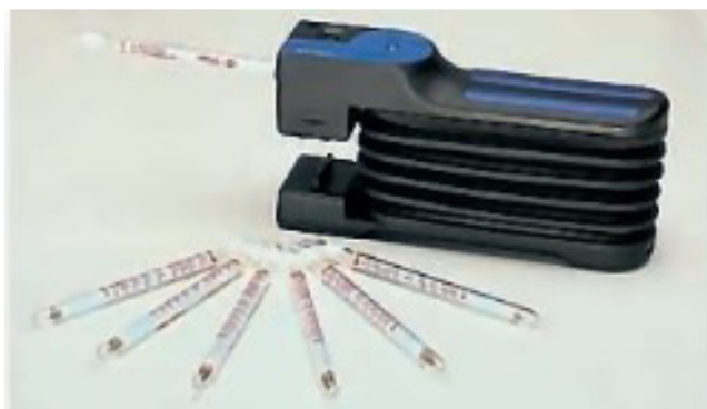
Figure 5. Local measurement of environmental ozone. Dräger ozone detector tubes and Accuro hand suction pump. Taken from ref. [4]
