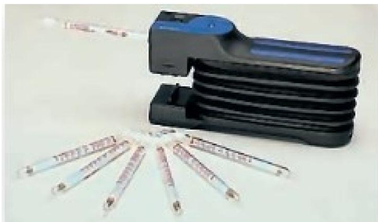
Figure 8.5. Local measurement of environmental ozone. Drager ozone detector tubes and Accuro manual suction pump. Taken from ref. [4].
