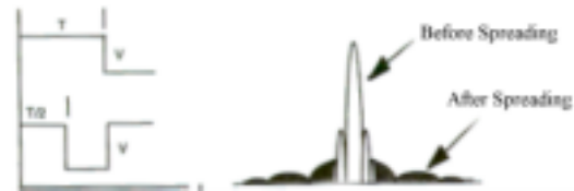
Figure 1 – Square pulse and power spectral density before and after spreading [2]
