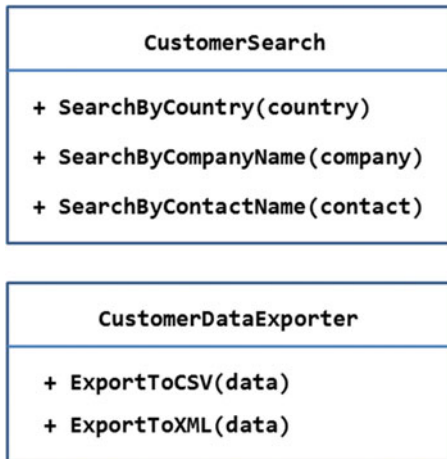
Figure 2-3. Class design after applying SRP
