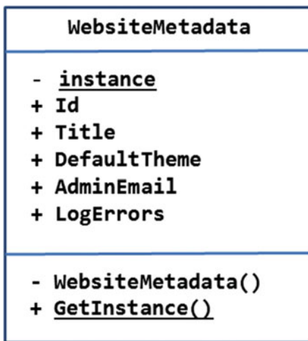
Figure 3-3. UML class diagram for WebsiteMetadata class
