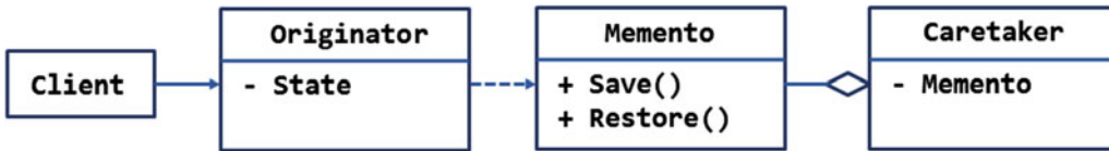
Figure 8-4. UML diagram illustrating the memento pattern
