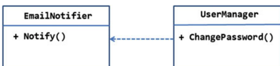
Figure 2-19. High-level class depends on a low-level class
