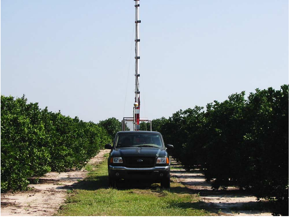
Fig. 2. Vehicle and trailer with vertical array of 10 ultrasonic transducers and DGPS used to measure tree heights and volumes. Transducers are mounted from 0.6 to 6.0 m above the ground.
