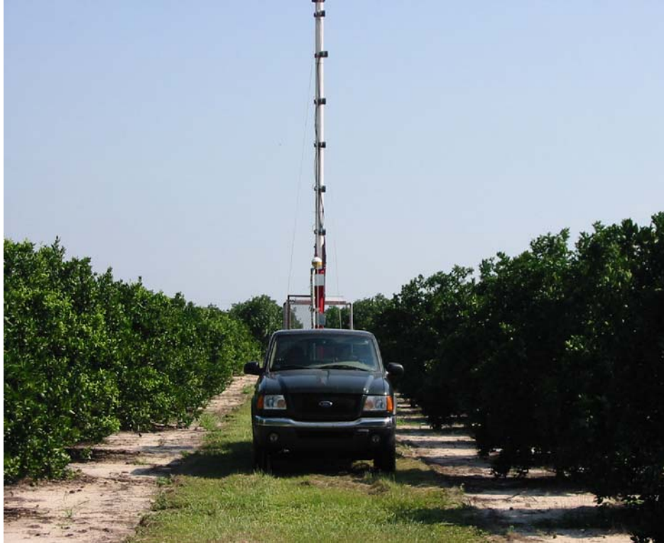
Figure 3. Vehicle and trailer with vertical array of 10 ultrasonic transducers and DGPS used to measure tree volumes.
