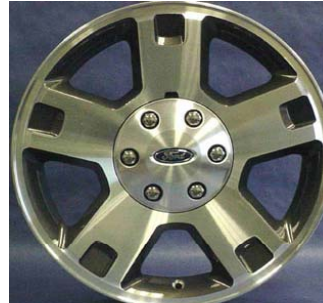
18" Machined Cast Aluminum (Opt. FX4) – (64L)
