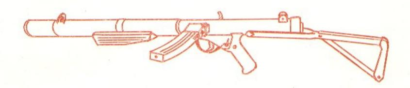
The Silent Sterling was designed to meet a requirement for a fully silent and very accurate weapon which would normally be used in "single shot". Under these conditions, heating of the external casing is not a problem that arises. However, under training sessions and demonstrations the casing can become hot to the touch.
