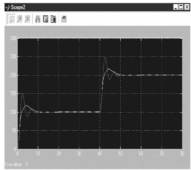
Figure 3 - Multi-Step Response for PID controllers tuned using GA and ZN (The process parameters are assumed to be time-invariant).
