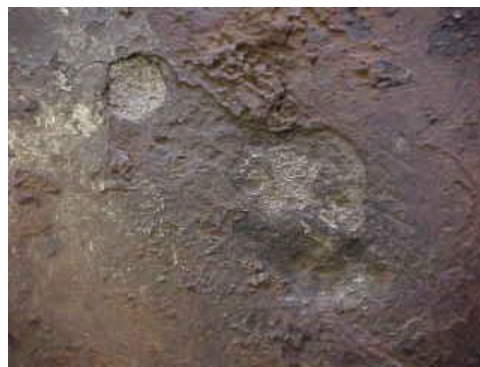
Sample 2 underside pitting
