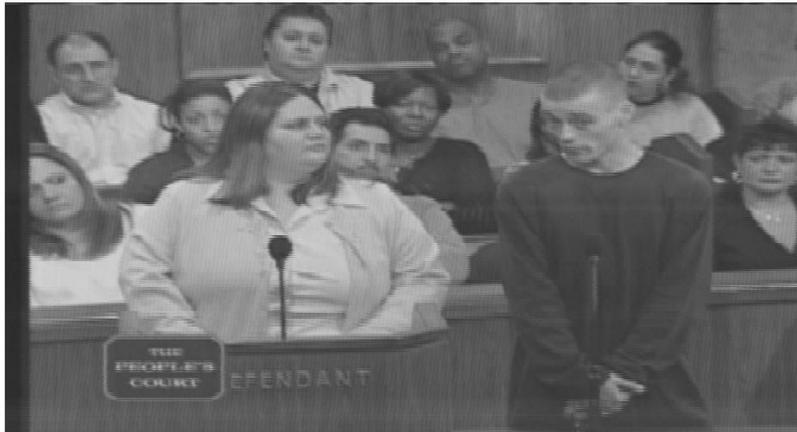
Figure 7.3: Luminance Image from an adaptive 2 line comb filter
