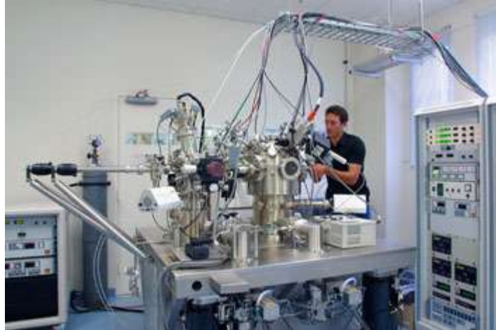
Figure 15 Customized combined STM-SEM system
