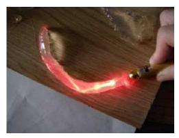
total internal reflection in a plastic "prism" and in a gelatin optical "fiber"
