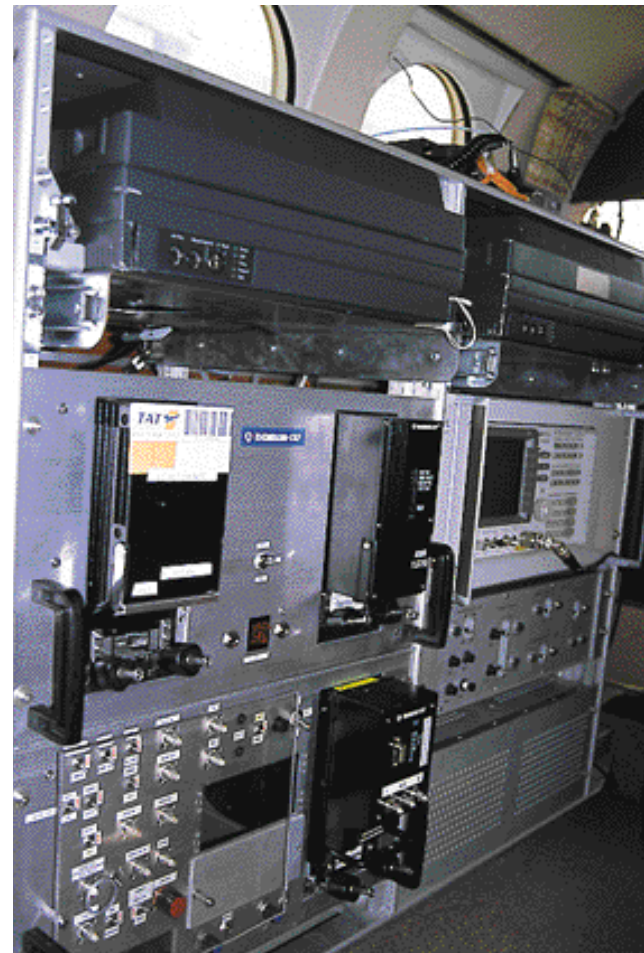
The bench, with a multi-mode radio running VDL 2, integrated onboard aircraft for flight-testing.
