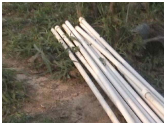
Plastic Threaded 1inch PVC “Drill Stem”
