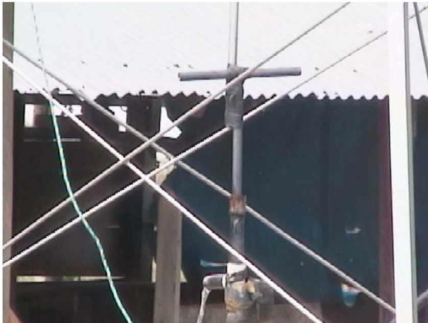
The above machine coupled directly to the pump handle with rubber inner tube. For quick pumping when no wind is available. Set up by user.
