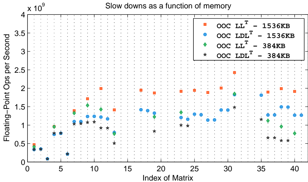
FIGURE 5.9. The performance of the out-of-core as a function of main memory size. The memory sizes shown in the legend are the target memory usage given to the code; the operating system itself had access to 2048 MB in one set of experiments and 512 MB in the other set.
