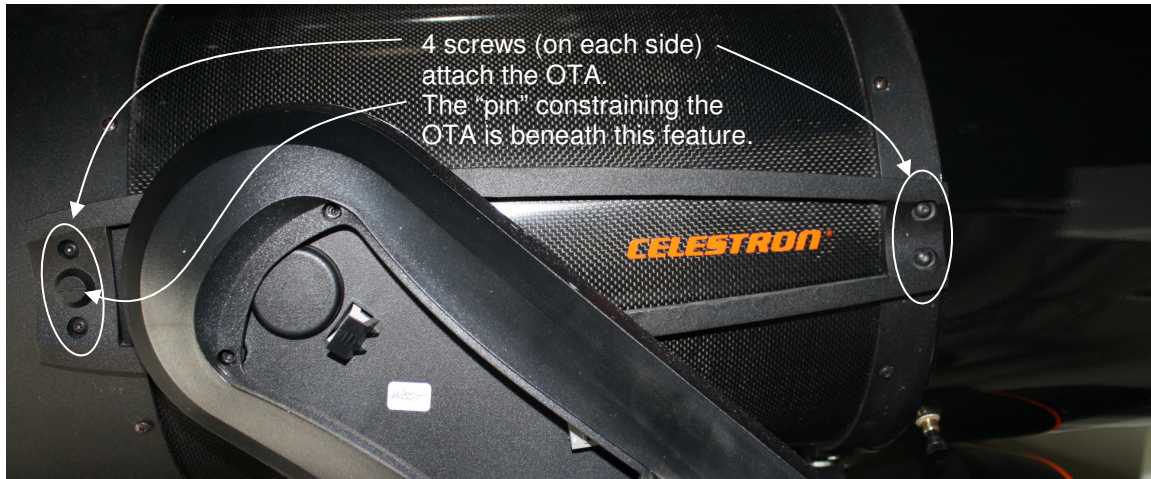
Figure 5: Bracket holds the Optical Tube Assembly
