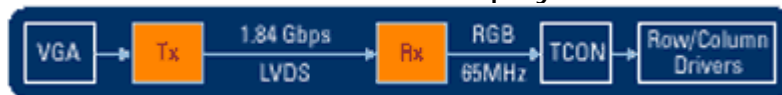
Figure 6. The LVDS FPD Link Moves Large Amounts of Data from the Notebook PC to the Display Panel
