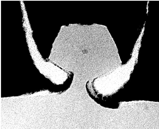
Cross-sectional TEM of a 4 nm Si quantum wire after stress-limited oxidation 1 .
