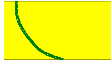
Useful Pattern to direct all fanout beams into single direction at the end of waveguide in an H-tree system (Curved guide has low loss compared with 90 deg waveguide)
