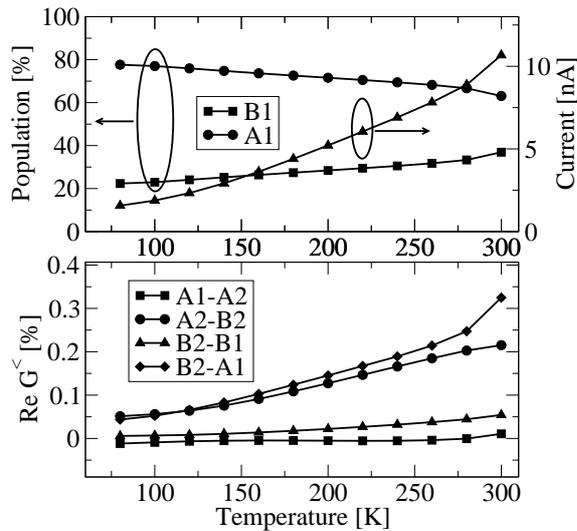
Fig. 3. Temperature dependence of populations of energy levels (top panel, left axis), current (top panel, right axis) and real part of coherences among states
