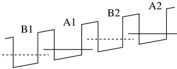
Fig. 1. Energy levels scheme of a QD cascade structure. Two periods of the structure.
